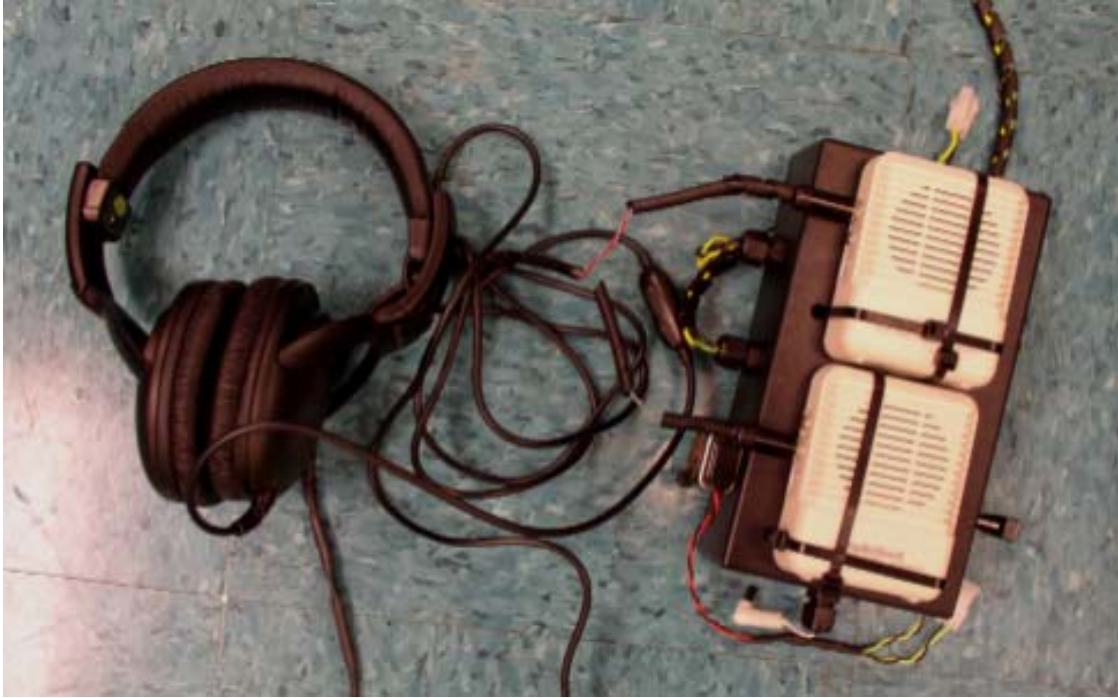
Stereo Hydrophone system headphones and amplifiers mounted on control box.
