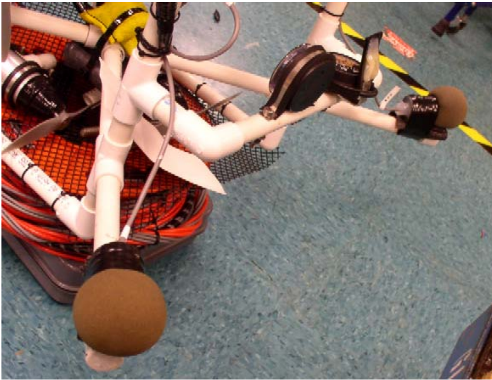
Dual Hydrophones mounted on Sea Perch frame, with foam covers.
